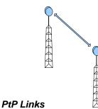
These use highly directional antenna to provide capacity between two fixed locations. They are very spectrally efficient and can provide very high data rates (up to a Gbps) and QoS (such as 99.999% availability).
