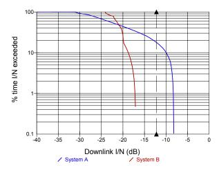
Here System A, which was nearer the equator than System B, experiences a worst case downlink I/N greater than the threshold of -12.2 dB (i.e. a DT/T = 6%).
