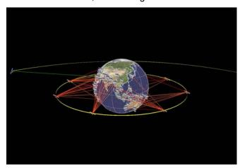
The figure also shows one of the key issues – the geometry involved. The O3B network satellites orbit at an altitude much less than that of the GSO.
