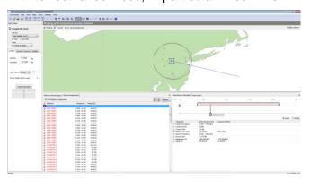
Visualyse EPFD: to determine if a non-GSO FSS system meets the EPFD limits in Article 22 of the Radio Regulations:
