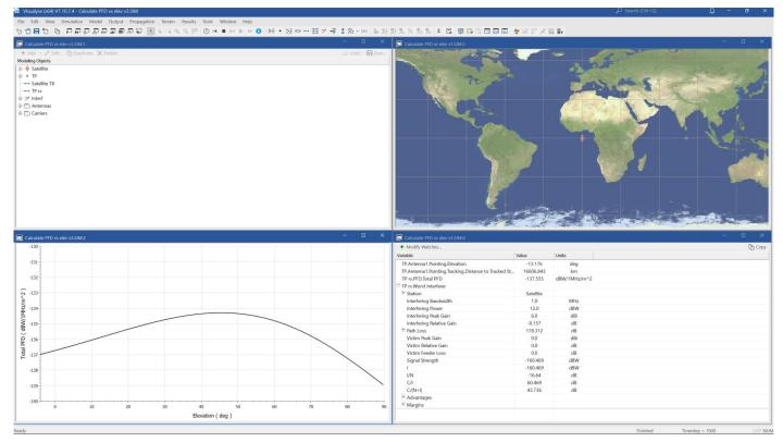
The PFD is measured at a test point that is located at the height of the ARNS receiver, namely 12.192 km. It is moved from the sub-satellite point to the edge of visibility, which for this height means the minimum elevation angle goes down to -4°. The satellite is modelled via the following parameters:
