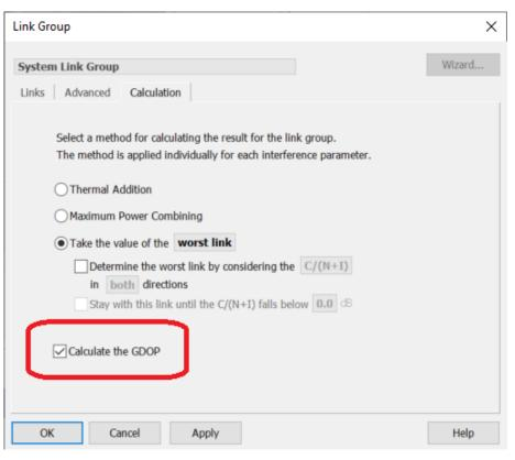
When selected, the GDOP is calculated over all the Links in the Link Group. For example, in this case, it would be calculated for 5 Links:
