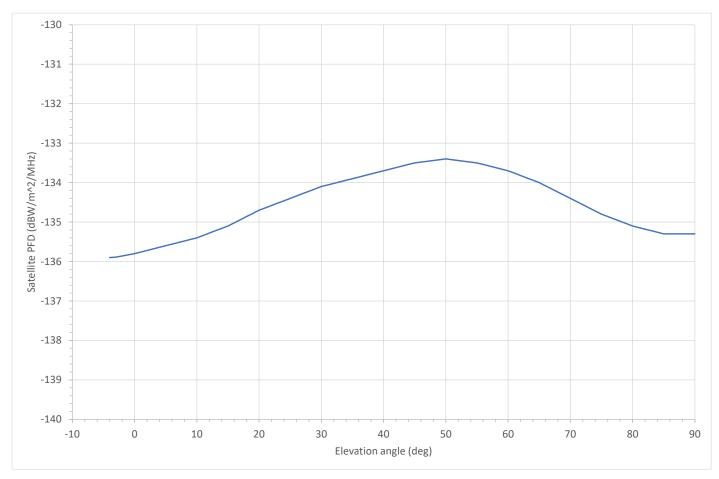
The satellite orbit parameters were read from the SRS for system GALILEO-2 and with a grid of test points the simulation was as shown in the figure below:
