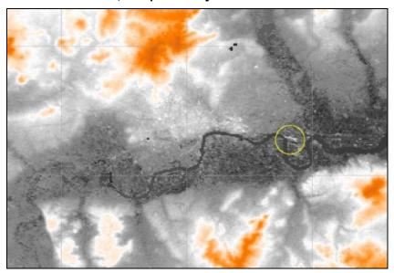
Additional features can be seen which include roads, railways, and buildings. The circled feature is the Docklands development to the east of London. It can be seen that there are structures in white, which are the large office towers, which are not shown in the previous OS database, which excludes surface objects like buildings.
