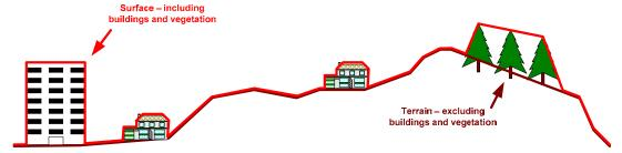
The figure below uses a surface database taken by radar from a Space Shuttle mission. It contains measurements of where the radar waves are reflected, which could be terrain but also be from structures like buildings sitting on the terrain. This data is freely available and can be downloaded from the USGS web site.
