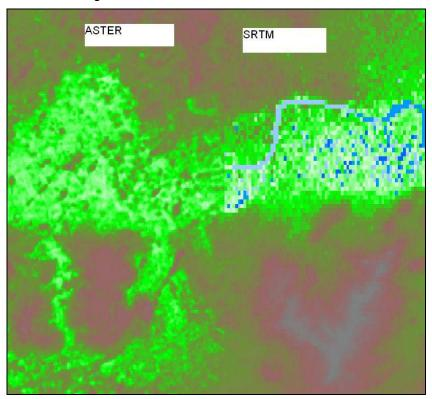
The SRTM is to the right and the Thames can be picked out. However on the ASTER data to the left while the pixels are small it is much harder to pick out this significant geographic feature due to the greater noise or variation in height at each pixel.
