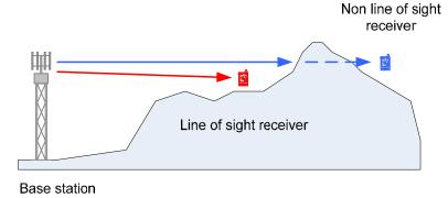
The base station is transmitting to two mobiles: the red one is in line of sight but the blue one is on the other side of a hill and so the signal will be reduced or attenuated due to diffraction loss.
