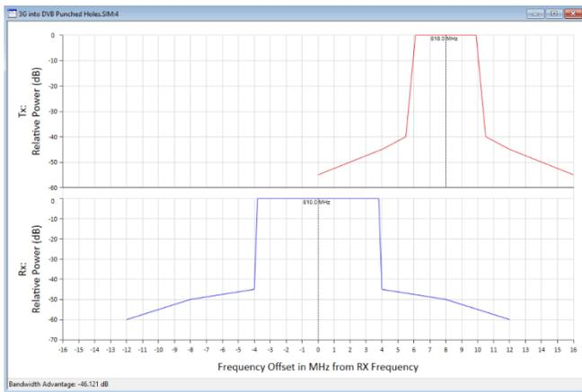
Note that the  $A_{MI}$  (i.e. the NFD) is shown in the bottom left of the view in the form that it is shown in the Watch Window, namely as the bandwidth advantage.
