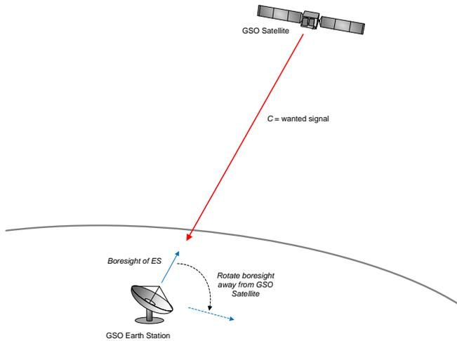
Here a GSO satellite with longitude = 0 is transmitting to a GSO Earth station at (latitude, longitude) = (0, 0). The ES antenna starts with pointing angle (azimuth, elevation) = (0, 90) and then the elevation angle is changed so that the antenna gradually points away from the GSO satellite.
