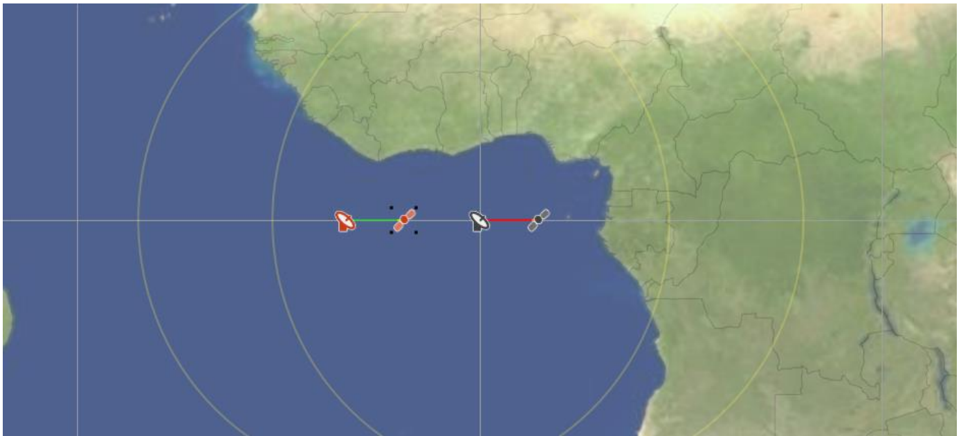
Figure 27: Screenshot of Doppler Example with Interfering Satellite between Two ES
