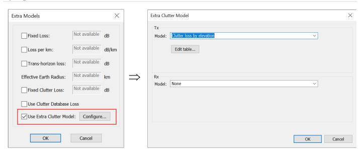
The clutter loss can then be entered for a set of elevation angles using a table like this:
