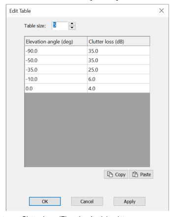
Linear interpolation is used between Clutter Loss (Elevation Angle) points.
