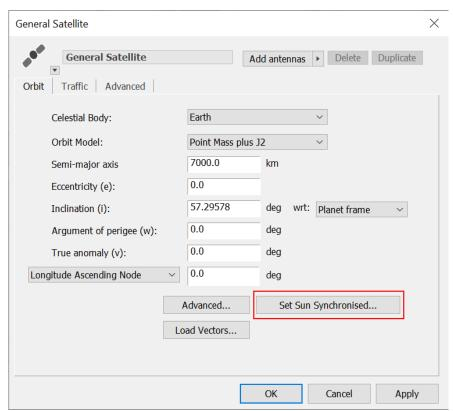
It can be used to configure a sun-synchronous orbit using repeating or non-repeating ground tracks:
