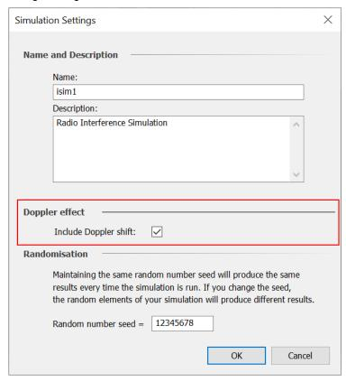
It is also possible to define the transmit or receive frequency so that it is adjusted to take account of Doppler shift on the wanted link:
