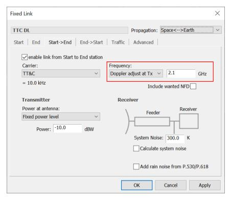
This can be done to keep the frequency constant at the transmitter or receiver and include the net filter discrimination (NFD) when calculating the wanted signal, if required:
