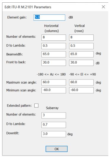
An alternative way is to define a set of Gain (azimuth, elevation) tables, one per skew angle. This option has been extended to allow any number of tables to be entered using the Advanced Beam Options controls here:
