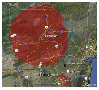
This picture shows the coverage in red of two US broadcast transmitters taken from the FCC database, namely a 200 kW ERP transmitter close to Scranton (fictional home of the US TV series *The Office*) and a 140 kW ERP transmitter at Springfield. Both are operating on channel 41 at 632 – 638 MHz.
