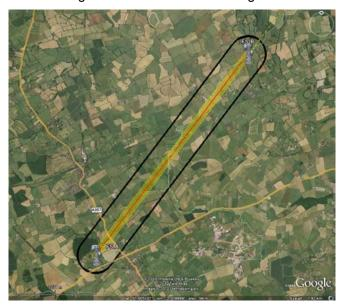
It was concluded that a 500m coordination zone should provide sufficient protection for links such as this.
