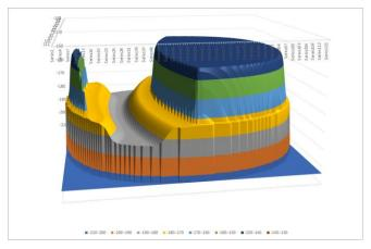
It is also possible to use the parameters entered to create a satellite EIRP mask.
