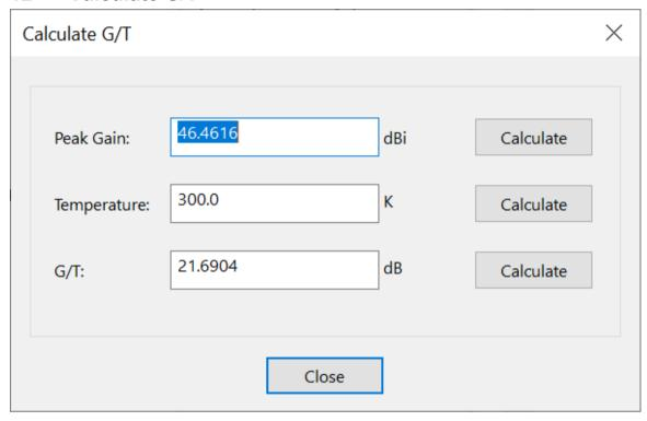
The G/T tool converts between peak gain and temperature in Kelvin to G/T. The following parameters are used:
