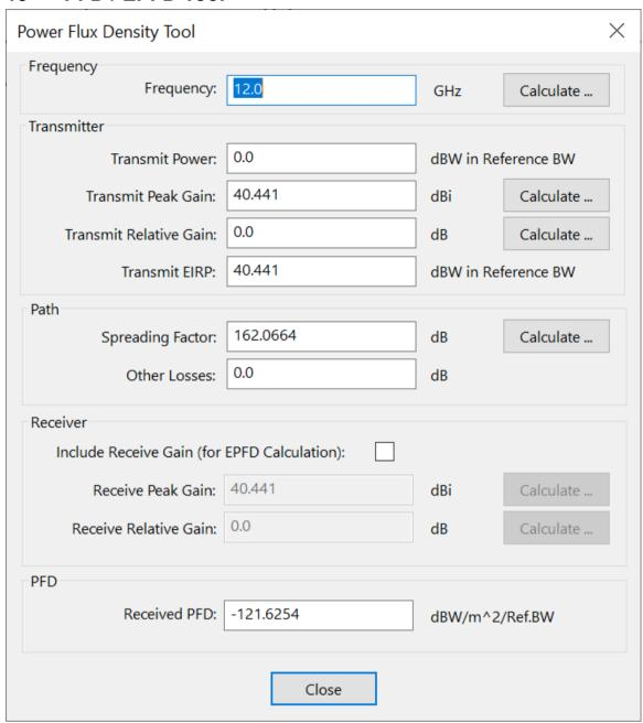
These various tools are combined to produce a PFD and EPFD tool with the following parameters:
