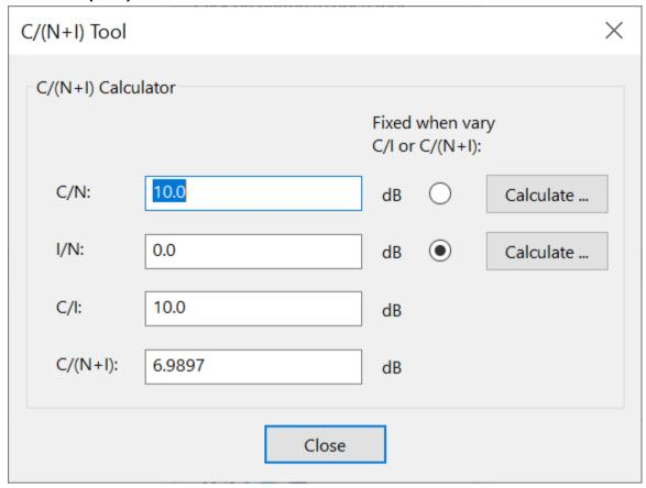
These tools can be used to calculate the link metrics  $\{C/N, I/N, C/I, \text{ and } C/(N+I)\}$ . In this tool the:
