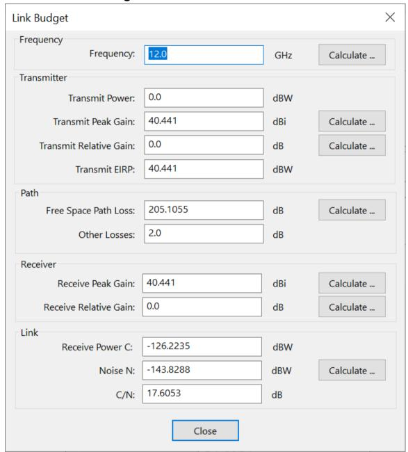
These various tools are combined to produce a link budget tool with the following parameters:
