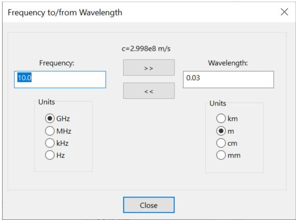
The Frequency tool converts between frequency f and wavelength  $\lambda$  using:
