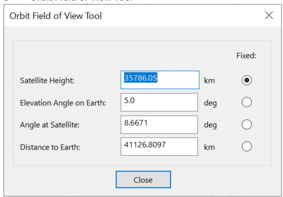
The angles tool provides information about satellite angles and distances. The parameters are:
