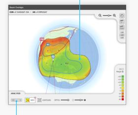
PLOT REOUIRED DISH SIZE. C/I, C/N, C/(N+I), ΔT/T, OFF-AXIS EIRP OR PFD
